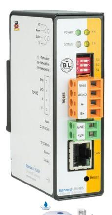
The Gateway connects Thies CLIMA sensor via RS485 to read the Modbus data points from the sensor. The sensor acts as a Modbus slave, providing data such as wind speed and temperature. Captured Modbus data points are mapped to BACnet objects, available via BACnet IP for building systems.
