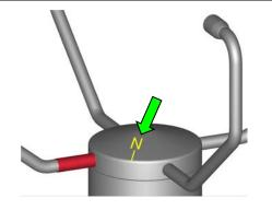
In the bottom of the anemometer stand there is a **north-drilling**.
